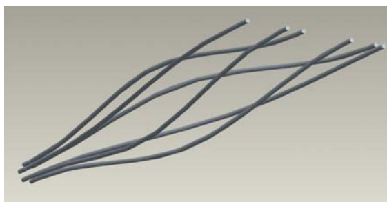
Concept design for a 3-dimensional integrated pupil remapping device for an astronomical telescope, consisting of a series of waveguides fabricated via ultrafast direct laser writing.
